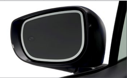
Auto-Dimming Exterior Mirrors with Approach Light. Designed to enhance nighttime driving safety by working in unison with the Auto-Dimming (Interior) Mirror to reduce headlight glare. Upon approaching the vehicle or unlocking your doors with the keyless entry system, LED lights in each exterior mirror illuminate the ground next to and towards the rear of the vehicle. Requires Auto-Dimming (Interior) Mirror.
