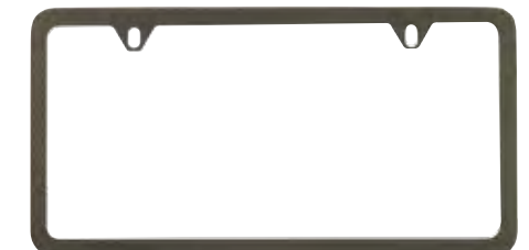
■ Slim Carbon Fiber License Plate Frame Carbon fiber composite license plate frame is hand made with thick resin-impregnated carbon fiber cloth, and is finished in a UV resistant clear coat. Kit includes hardware hider caps. SOA342L142
