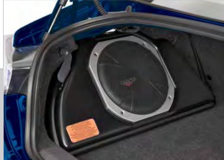
■ 10 Inch Powered Subwoofer Provides powerful deep bass, and also assists in a clean sound reproduction from all vehicle speakers. This is achieved by its integrated 100W amplifier and a passive crossover network. The self-contained unit mounts in the trunk of the vehicle. Manufactured for Subaru of America by Kicker®. H630SCA000 Cannot be installed with Cargo Tray.
